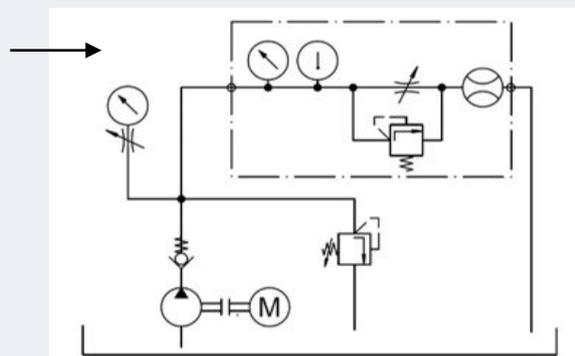
Figure 9: Hydraulic diagram of pump test
