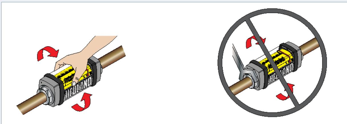
Turn the volume flow meter by hand so that you can see the flow scale.
