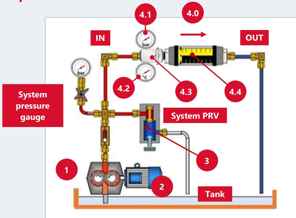
Figure 8: Schematic diagram of pump test
