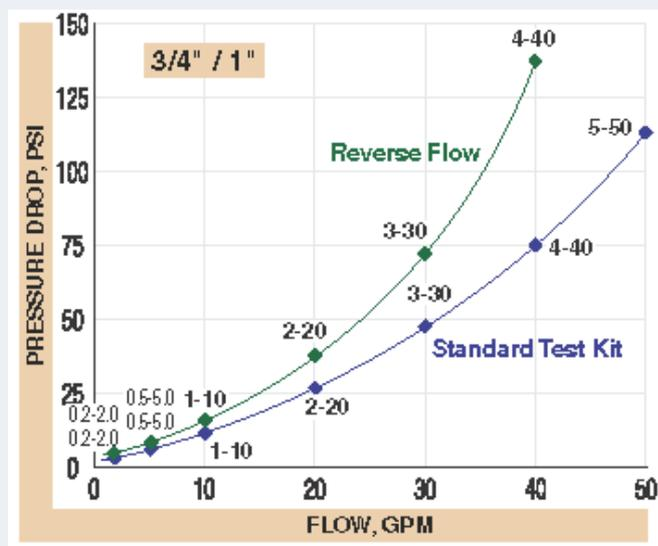
Graph 1: p/Q characteristic curve for pressure drop (blue) for a standard ¾" and 1" power meter
